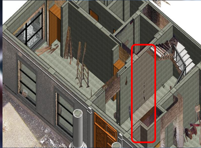
As Per BIM Model No Opening
